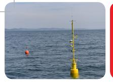
Under water detection and positioning system is a mobile system used to accurately detect, monitor and track the positions of surface and underwater platforms for qualification purposes. It also can measure the acoustic fingerprints of the platforms.
