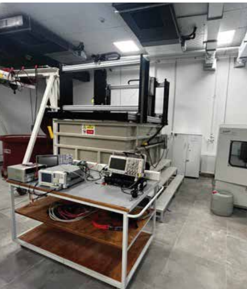
Climatization Cabinet and Pressure Tank
